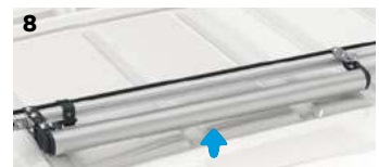
Space Up roof rack roller F22UP0606100000 W= 615 mm for Connect / Custom F22UP0607800000 W= 780 mm for Connect / Custom F22UP0609500000 W= 950 mm for Connect / Custom
