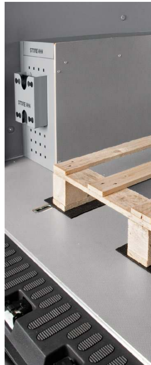
Anti-slip mats are used to increase the coefficient of friction up to \mu_D 0.6 in accordance with the calculation principles of DIN EN 12195-1:2004 and VDI 2700 ff. Measurement procedure according to VDI 2700-15.
