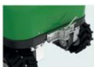
Attacco traino. Towing Hitch.
